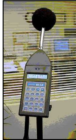
Sound meter of the type used to measure noise levels for this General Plan
